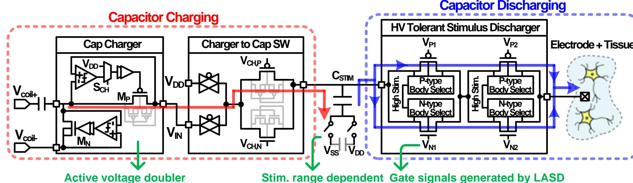
☺ Cap. charged through active diode : high charging efficiency
